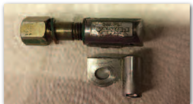
Broken pressure reducing valve
