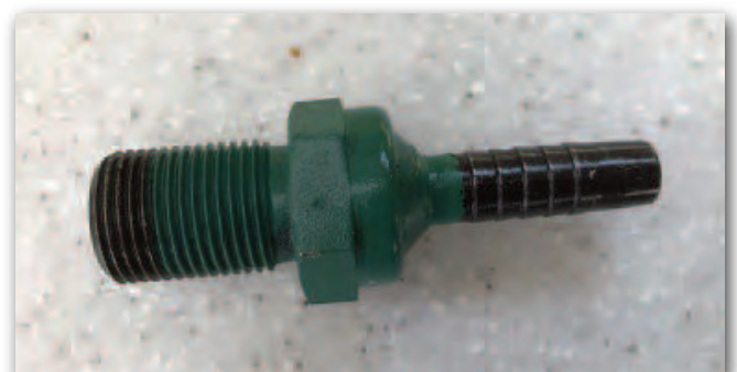
Blocked or seized non-return Valve
